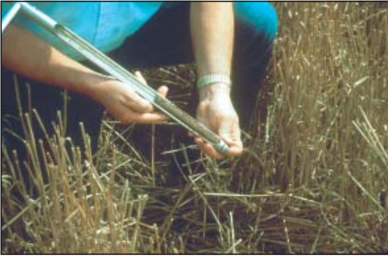
Consistency in depth of soil samples and lab procedure used is important in monitoring long-term changes in soil organic matter levels.
