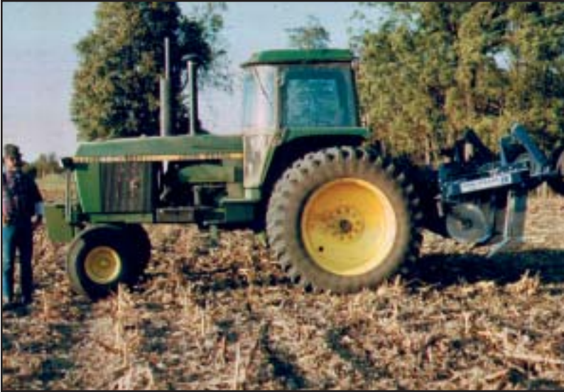
There are many types of “vertical” tillage tools which when properly operated cause minimal soil surface or residue disturbance. All tend to “heave the soil up and set it back down.” These tools may aid in the transition to no-till as macropores develop or may be needed every 2-3 years on certain soil types.
